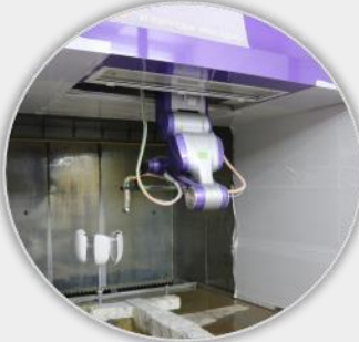
Robotic operated paint shop
